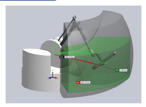
The Virtuose 3D Desktop is composed of two main articulated segments fixed on a rotating base. The second segment ends with an articulated wrist, which can rotate around three concurrent axes. As a consequence, the haptic interface is a 6 degrees-of-freedom device, with force-feedback on the 3 first axes. The structure of the Virtuose 3D Desktop can work in a volume corresponding to a torus with a square section of 20 cm. The center of the square is 30 cm from the base of the device.
